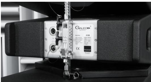
Galeo S units, stacked on a subwoofer via Galeo S Stacking Board
