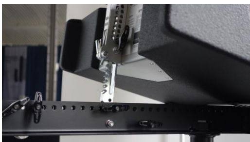
Galeo S unit, mounted on a Galeo S Flying Cradle with maximum down-tilt
