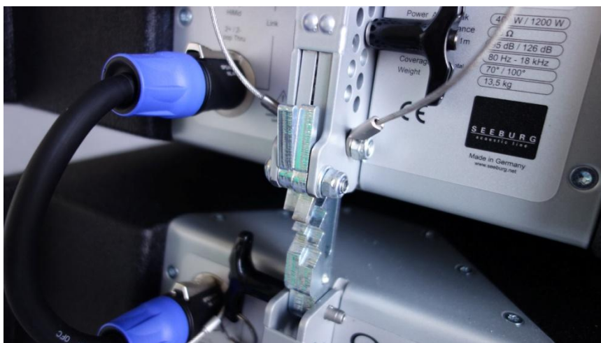
Checking that all of the Auto-Locking Hooks have locked in correctly
